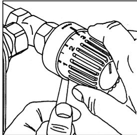
1. Remove the handgrip with the tool (item no. 198 91 00) or with a pin, e.g. with the push button of a pen. Insert the tool/pin in the hole on the bottom of the thermostat. By turning the handgrip into the shut-off position, it is easily removed. After having removed the handgrip turn the knurled screw to the left until the red calibration mark is in line with the indicator mark.
