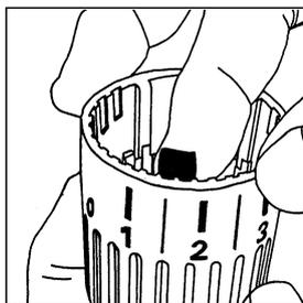
3. To limit the minimum temperature range, e.g. to position "2" (corresponds to about 30 °C), one clip should be fitted into the groove immediately **before** position "2" as illustrated. (The groove directly in front of position "2" thus remains free.)
