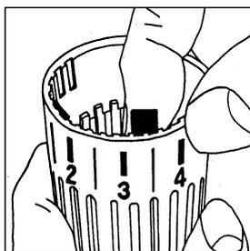
4. To limit the maximum temperature range, e.g. to position "3" (corresponds to about 40 °C) the second clip should be fitted into the groove immediately **after** position "3". (The groove directly in front of position "3" remains thus free.)
