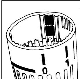
2. Inside the handgrip you will find two clips in the "parking" position as illustrated. They can be removed by sliding them to the outside. (If the clips are not used, they can of course be stored in the "parking" position.)
